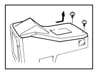
2 Remove the Power Unit Cover. (3 screws)
